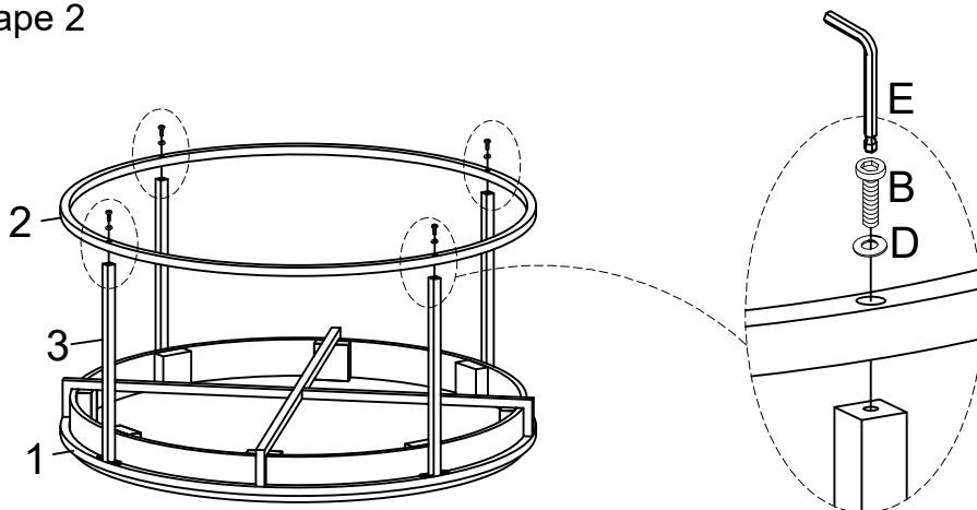
**Note: At this stage, tighten all Bolts at all joints fully in a sequential manner.**
